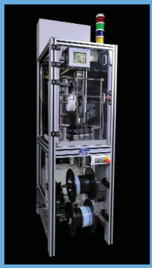
Material is wound on specialized Steeger machine.
