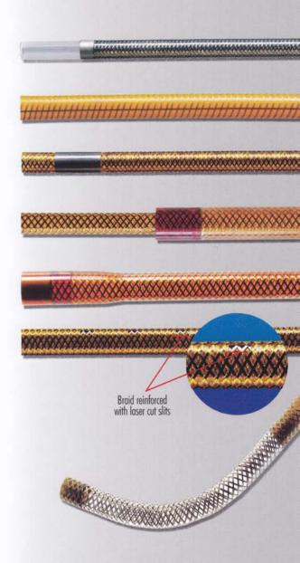
MicroLumen offers custom braid and coil reinforced tube shafts. The primary advantages of reinforcement include increased column strength, torque transmission and increased burst strength. Reinforced tubes are available in a wide range of diameters and configurations.
